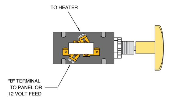
Mount the Heater switch in a 7/16 inch hole.
